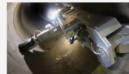
CISBOT innovation - (Cast Iron Sealing Robot)
